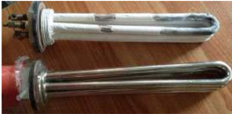
Figure 1. An autoclave water-heating coil covered with a layer of deposits (most likely to be CaCO 3 from hard water) and a newly purchased heating coil (picture taken in one of the hospitals included in this study).
